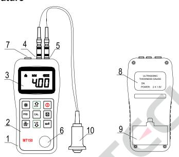
1 The main body 2 Keypad 3 LCD display 4 Pulser socket 5 Receiver socket 6 Probe zero disc 7 Communication port 8 Label 9 Battery cover 10 Probe
